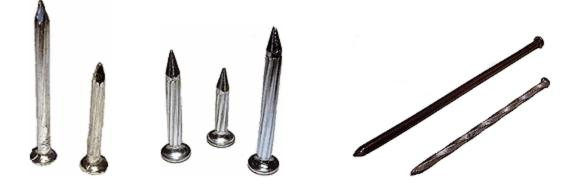
The most common anchoring device is the nail. For tarmac roadways you would use tarmac nails, masonry nails, or PK nails. For soft shoulders you would use spikes which come in a variety of lengths from 150mm (6 inches) to 300mm (12 inches) depending on the firmness of the shoulder. You will need a pretty hefty hammer for driving in the nails or spikes. In tarmac, you can also use power nails and an anchor plate with a portable nail gun (not common, but quick).
