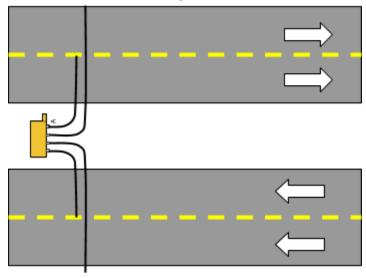
This is a volume only configuration that also allows you to count occupancy in four lanes. Though shown in two directions in the setup above, the lanes can all be in the same direction. This configuration has less error in the long hose counts since they only encompass two lanes.
