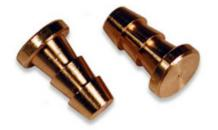
Commercial brass end-plugs. These devices are barbed and just press into the end of the hose. You have to specify what size center hole they are designed for. These can be purchased with a pin-hole for hot temperature use. These are high cost, more so when a pin-hole is needed.
