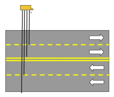
This is a volume only configuration that allows you to count occupancy in four lanes. Though shown in two directions in the setup above, the lanes can all be in the same direction. Again, in high volume situations, the three longer hoses will tend to count low when there are simultaneous hose hits in more than one lane at a time.
