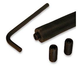
Commercial threaded end-plugs. These devices are threaded like the bolts mentioned above, but use an Allen drive to thread them in. They are made of stainless steel. They do not have the big head of the hex-head bolt, so present less of a hazard should they come loose on the roadway. You must specify what size center hole you will be plugging. These are of moderate cost.
