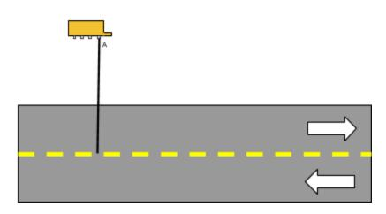
In this configuration volume only data is collected. In the hose setup screen you can specify the direction of the traffic being counted. The single hose may be connected to any of the four available input nozzles, however, to insure the least amount of problems at data interpretation time, you should always use the same nozzle (A,B,C, or D) for all your single hose data collection.
