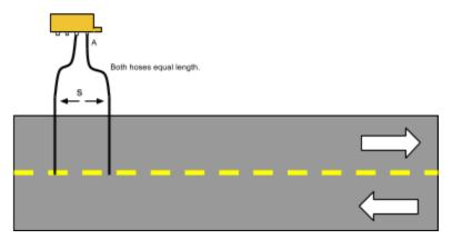
This hose setup is the normal configuration for collecting speed and classification information from one lane. In order to gather speed and classification data, you need two hoses.
