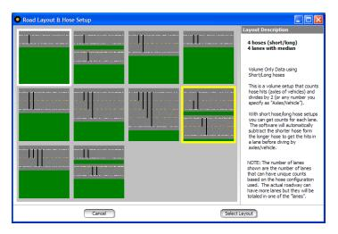
Highlight the hose setup that best represents how you had the hoses set up for the study then click on "Select Layout". In this example, we were collecting volume data from a four lane road with a median, two lanes travelling North and two lanes traveling South, using a long hose - short hose scheme for each side to allow us to get occupancy of all four lanes. This is the eighth layout (shown highlighted).
