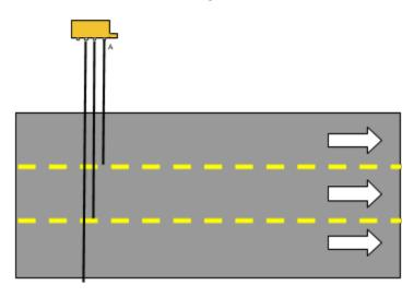
This is a volume only configuration that allows you to count occupancy in three lanes. Though shown in the setup above, the lanes do not all have to be in the same direction. Again, in high volume situations, the two longer hoses will tend to count low when there are simultaneous hose hits in more than one lane at a time.
